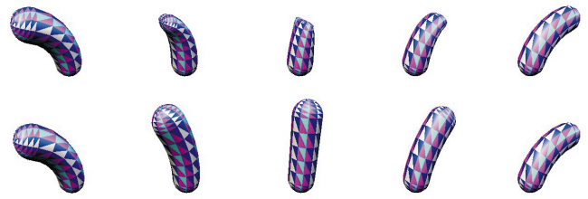
Figure 14: A simple example of three-dimensional objects. The difference of linear and as-rigid-as-possible vertex interpolation is demonstrated on a bent cigar-like shape.
